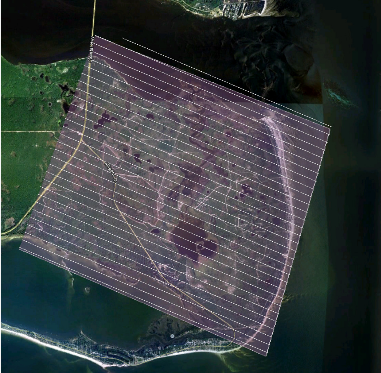
Figure 3. Project area of interest and planned flight lines.
