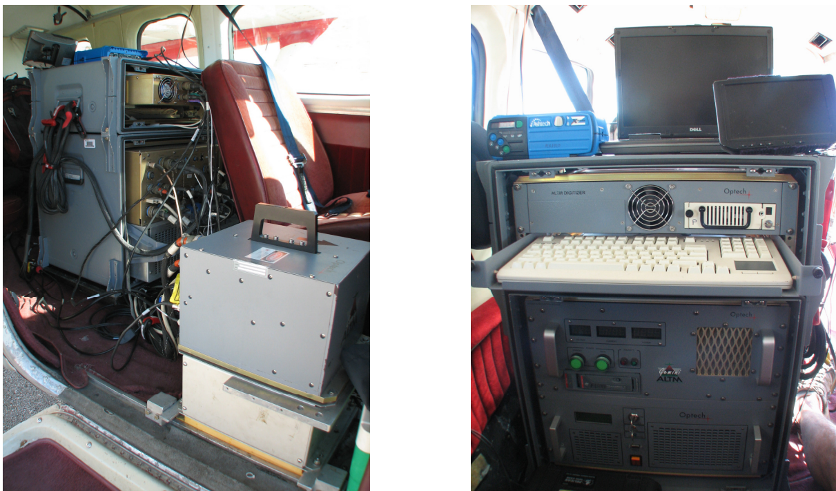
Figure 1 – NCALM Gemini ALTM installed in the Cessna Skymaster N337P.
